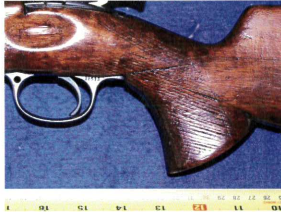
Figure 2 – Pistol grip and stock showing possible alteration marks
