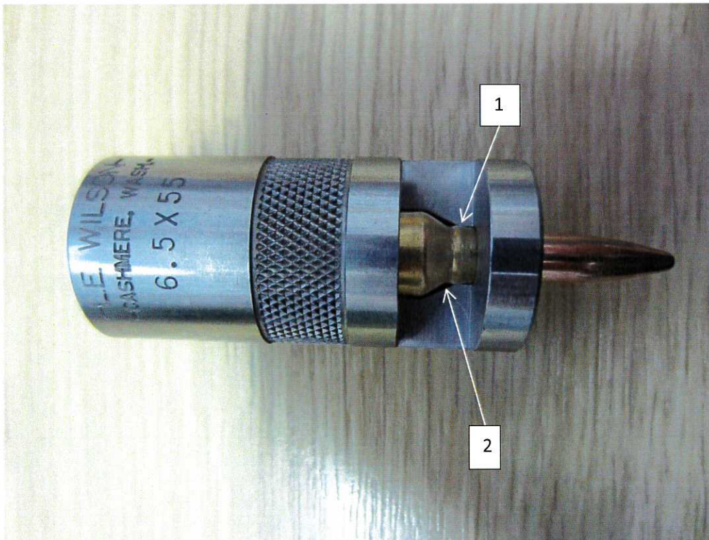
Photograph 7 – Round of ammunition from ammunition box, inserted in a case gauge, which mimics the shape of the rifle chamber. Note the bulge in the neck of the case (1) preventing the shoulder of the case (2) from contacting the gauge.
