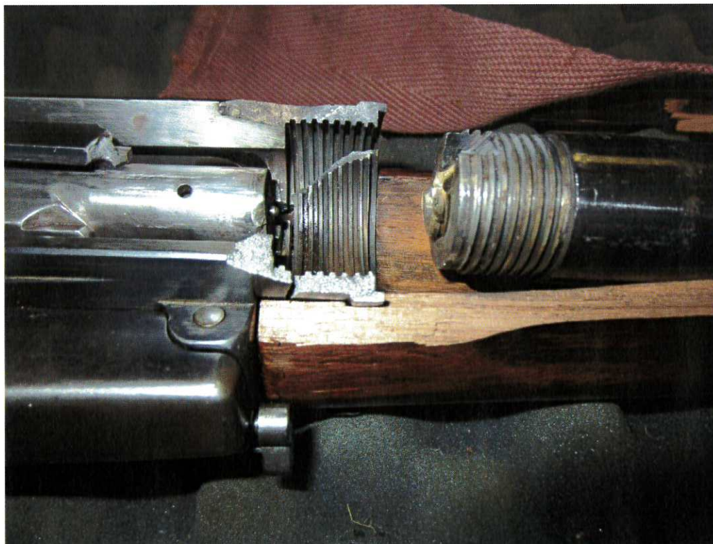
Photograph 4 – Krag-Jorgensen rifle after the accident. Two parts of the receiver ring in the centre of the photograph, broken end of the extractor upper left, barrel with ruptured case in the breech right.
