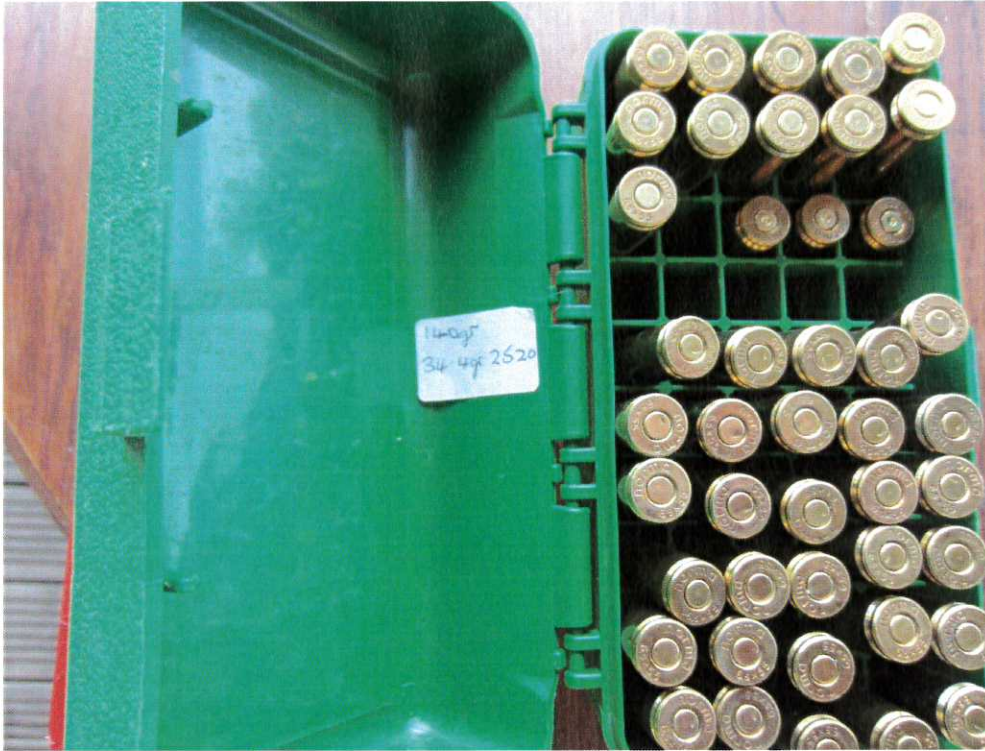
Photograph 6 – ammunition box showing live rounds and fired cases recovered after the accident, and label indicating the bullet weight and powder load.
