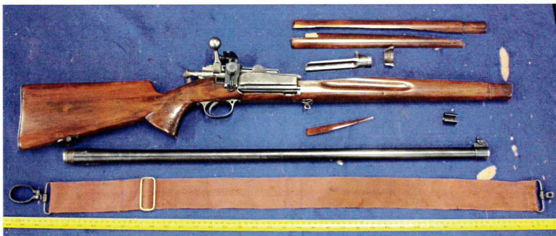
Figure 1 – Submitted components of a Krag-Jorgensen rifle
